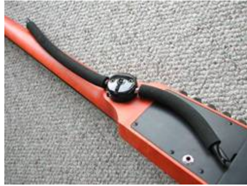
Folded for Storage For storage, move the long arm toward the neck, and rotate the short arm back over the body
