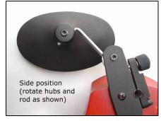
Height of the chin rest can be lowered by reversing the inner hub so it is on the bottom side of the attachment plate. Thicker washers can be used to raise the chin rest.
