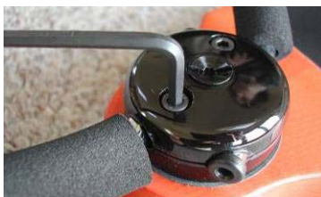
Adjusting Long Arm Friction
