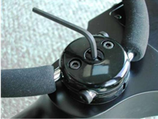
**Attachment to the Instrument** - The large, thin washer should be placed between the instrument and the hub (failure to use the washer can damage the surface of the instrument). Insert the attachment screw into the threaded insert on the back of the instrument. Use a 4 mm hex wrench, flat screwdriver, or coin to tighten the screw. The hub should be held firmly but still be able to rotate.
