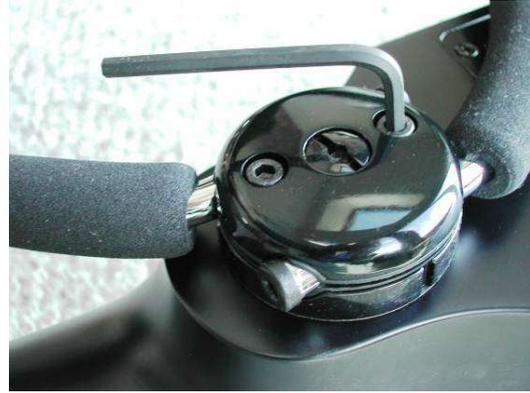
**Adjusting Pivot Friction** - To adjust the arm friction, tighten or loosen the two hex screws in the hub. The screw closest to the long arm should generally be tightened more than the other screw, to provide more friction on the long arm. The hex wrench can be stored in the hole in the ends of the tubes, but care must be taken to insure that the hex wrench is not positioned where it will scratch the instrument when the arms are moved.
