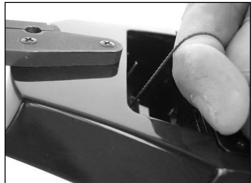
Pre-tension Synthetic Core Strings
