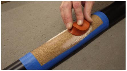
4. Continue sanding until the thumb stop conforms to the shape of the neck. This may require more than one sheet of sandpaper.
